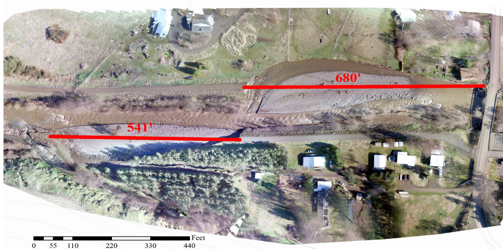
Milton-Freewater Levee failure. Destroyed levee centerline in red. (Walla Walla Basin Watershed Council, 2020)
